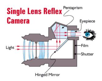
When you press the button on an SLR camera, the mirror flips up exposing the film to the light coming through the lens.
